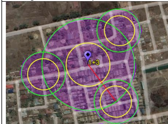
One Base Station and 3 Satellite APs Coverage Area: 117,000 sqm
